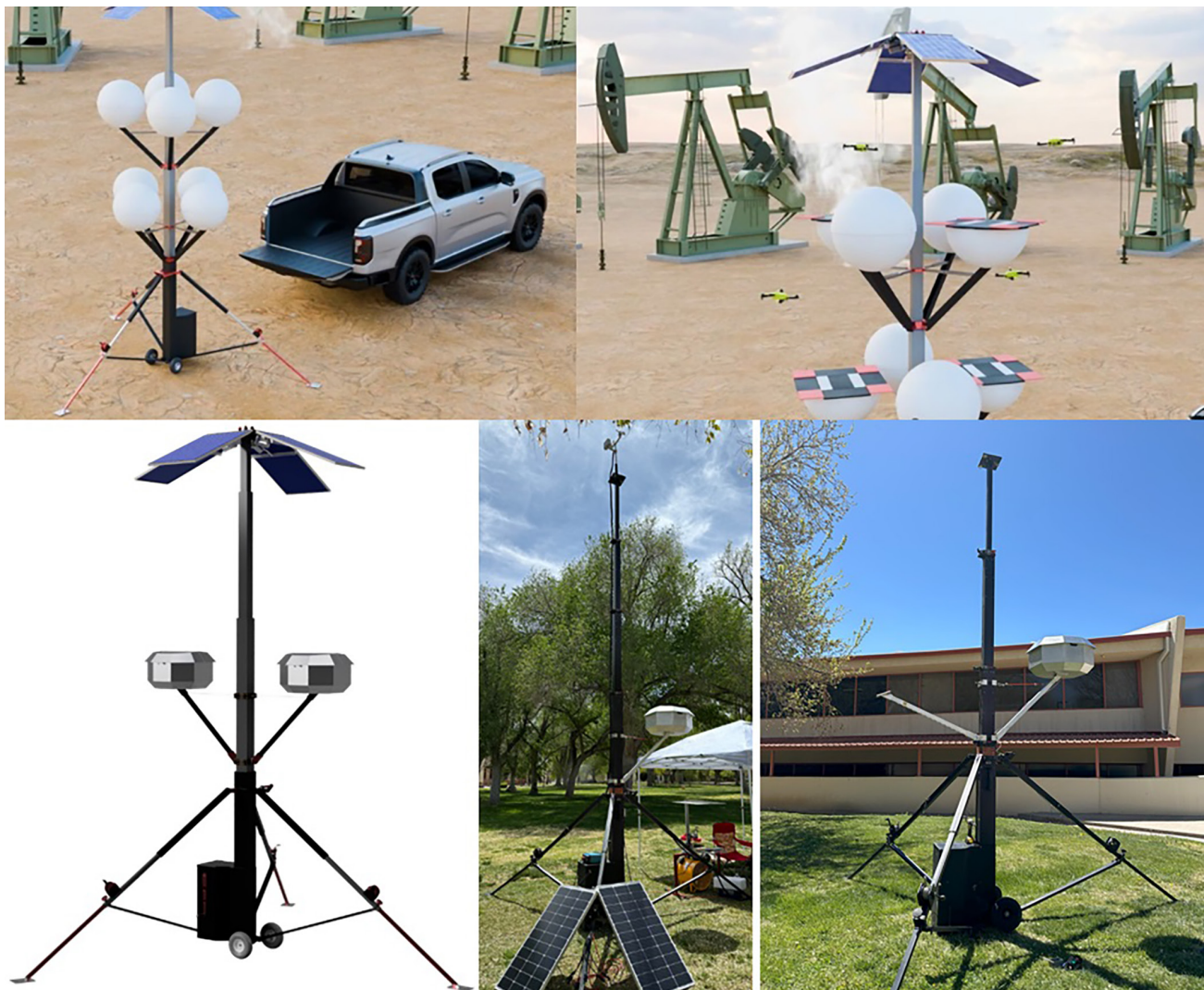
Figure 10. Proposed concept and current prototype of the vertiport.
