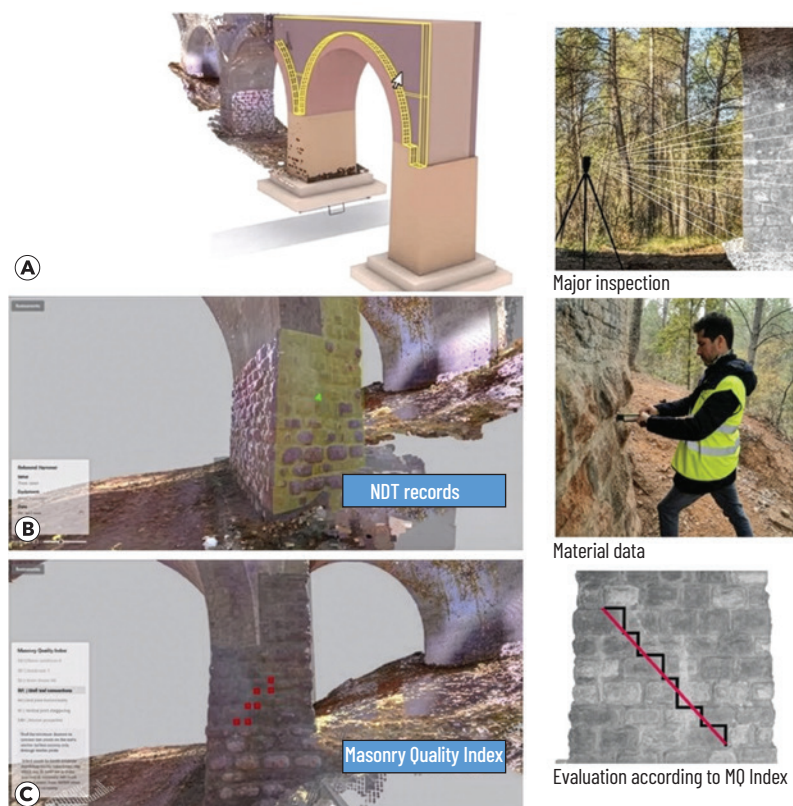
Figure 8. Systematic twinning of geometrical, material, and assessment data for a set of similar existing masonry bridges that exceeded their nominal service life: (a) scan-to-BIM geometric twin generated from laser-scanner point clouds and transformed into IFC objects using MatchFEM; (b) NDT and MDT material data linked to the 3D model via georeferenced records; (c) structural evaluation using the Masonry Quality Index (MQI), with results mapped onto the twin and assessed through standardized indicators.
