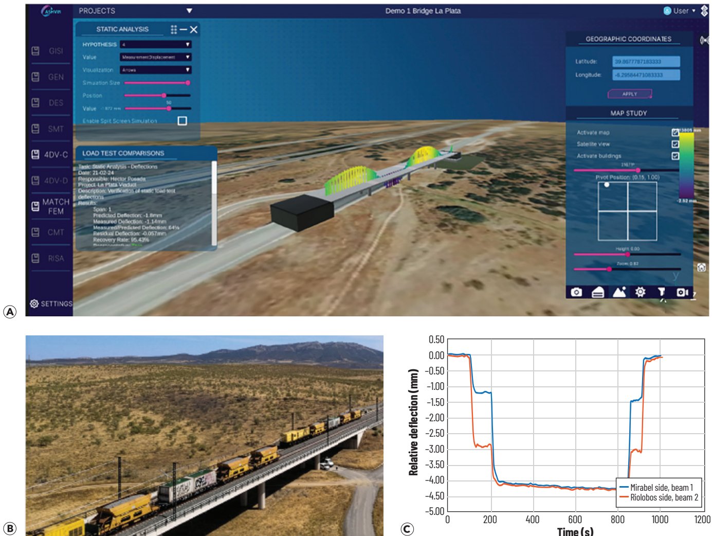
Figure 6. Connection between load test and digital twin: (a) dynamic analysis results visualized in the bridge digital twin; (b) static load test with comparison of measured and predicted structural response; (c) measured deflections during load test.
