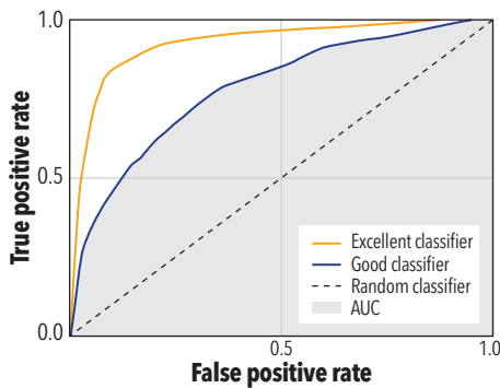
Figure 6. Receiver operating characteristic (ROC) curve. The ROC curve is achieved by plotting the false positive rate versus the true positive rate at each classification threshold. The quality of the ROC curve can be summarized by the area under the curve (AUC) shaded in gray.
