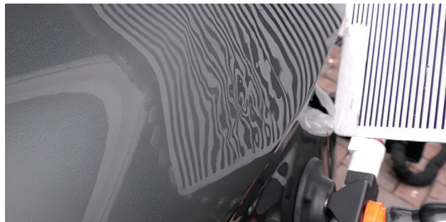
Figure 8. Using a visual aid for determining the extent of the dent.
