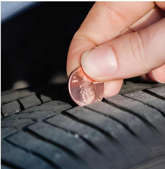
Figure 1. Measuring tire tread depth with a Lincoln penny.
