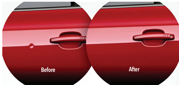
Figure 9. A dent repaired using PDR.
