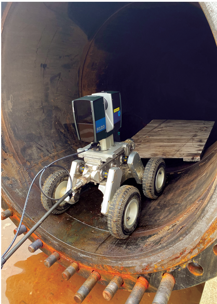
Figure 3. Crawler equipped with a 3D laser scanner. Also note the “bridge” utilized to drive over the exposed tee connection at the bottom of the line.
