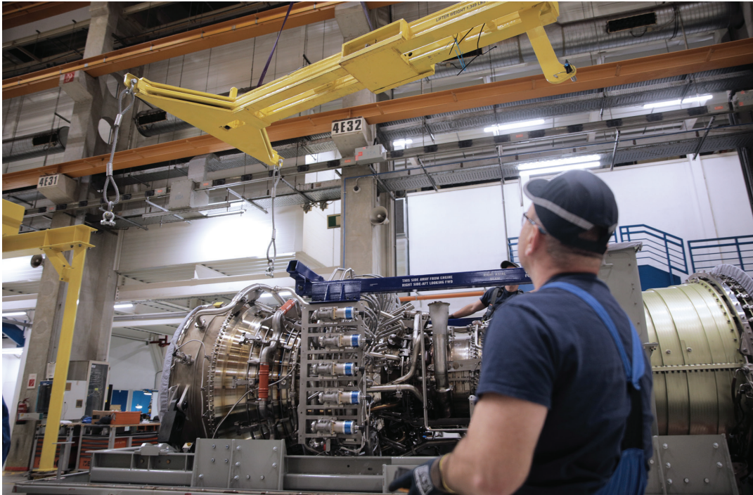
Figure 3. GE Vernova readies an LM6000 aeroderivative turbine for service.
