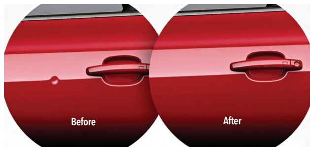
Figure 9. A dent repaired using PDR.
