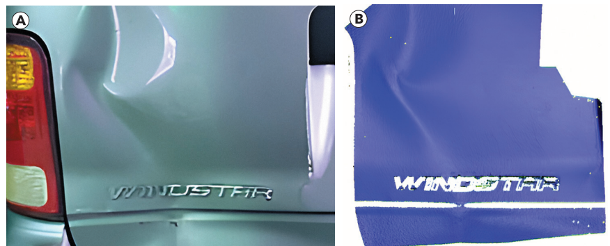
Figure 10. A structured light system for imaging dents.
