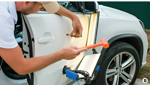
Figure 7. Dent repair: (a) Pulling and (b) pounding the dent.
