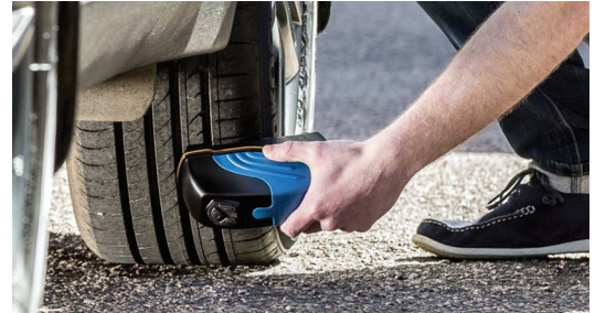
Figure 5. Laser line scanning system.
