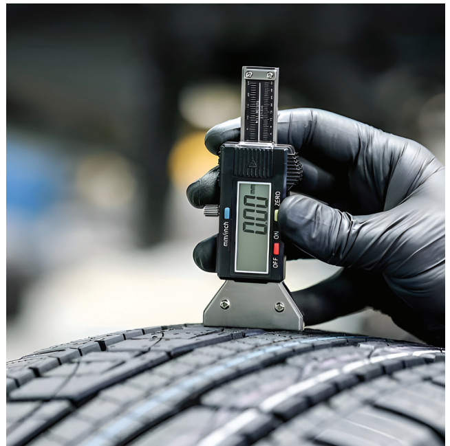
Figure 2. Measuring tire tread depth with a depth gauge.
