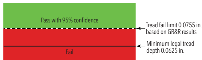
Figure 3. The impact of a visual inspection on the tread depth fail limit.
