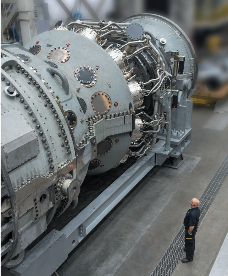
Figure 5. Large frame 7HA.03 GE Vernova gas turbine.
