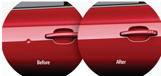
Figure 9. A dent repaired using PDR.
