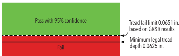
Figure 4. The impact of a machine vision system on the tread depth fail limit.
