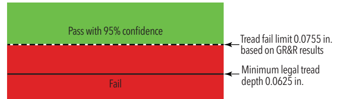
Figure 3. The impact of a visual inspection on the tread depth fail limit.
